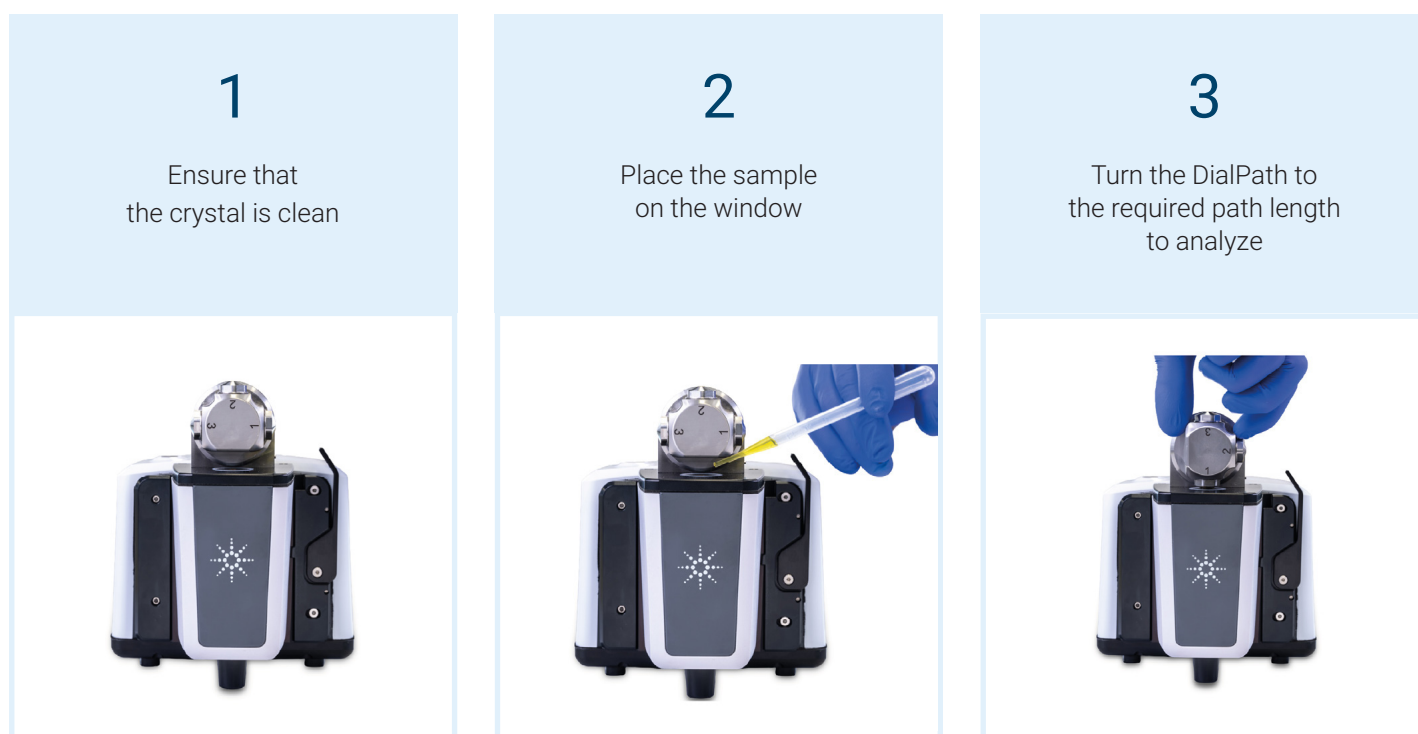
Figure 2. Three easy steps to analyzing liquid samples with the Agilent Cary 635 FTIR.
